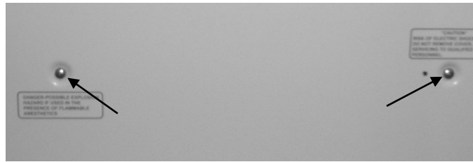
Figure 4 – Middle Rear Panel Screw Locations
